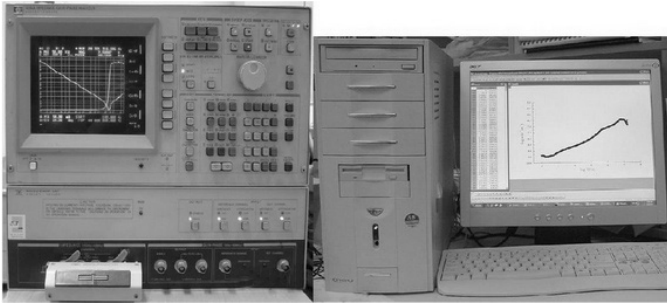
Fig. 1. A sophisticated computer controlled AC-impedance system.
