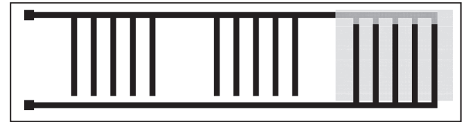
Figure 8. Behaviour of designed IDC in the case of positioning with complete match of electrodes, with paper as a dielectric.
